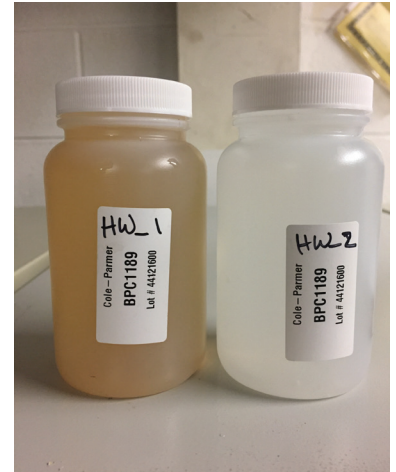
Water samples collected directly from water heater drain. Initial draw pictured on the left.
