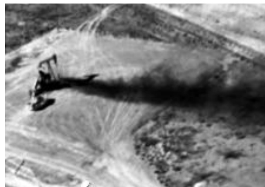
Infrared footage reveals significant methane emissions from a pump jack in the Permian Basin
