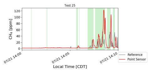
**Figure 2.11. Example Test Data from 300-scfh Release for the Point Sensor** The green bars represent periods in which the wind generally was directing the released gas towards the technology. The measurements from this technology aligned well with the reference measurements.
