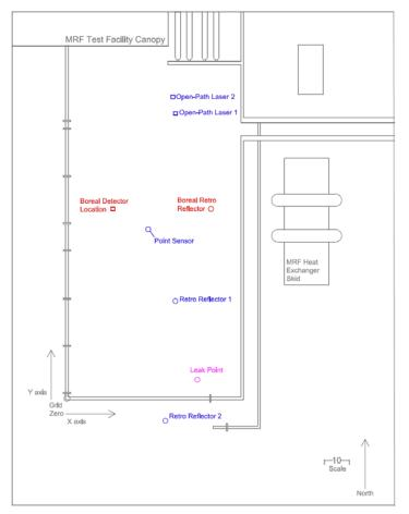
Figure 2.10. Location of Leak for the Data Analyzed in this Section The data analyzed include several methane releases from a single leak point.
