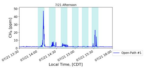
Figure 2.8 Readings from Open-Path #1 Over the Course of One Afternoon The blue bars represent periods in which leak tests occurred.
