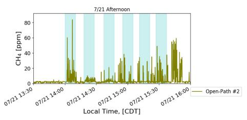
Figure 2.9 Readings from Open-Path #2 Over the Course of One Afternoon The blue bars represent periods in which leak tests occurred.
