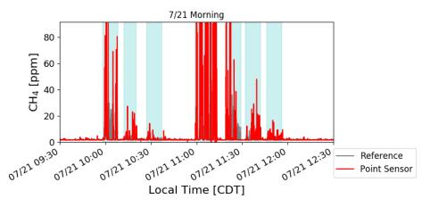
**Figure 2.14. Measurements from a Point Sensor** This plot has the same scale for both the reference TDLAS system and the point sensor.
