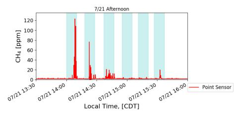
Figure 2.7. Readings from the Point Sensor Over the Course of One Afternoon The blue bars represent periods in which leak tests occurred.
