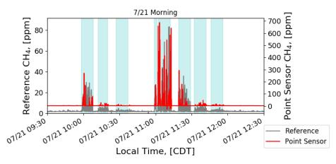
**Figure 2.15. Same Figure as Previous Plot with a Secondary Scale** This plot shows a significant difference in readings between the two instruments. However, the fact that one is a point sensor and the other an open-path device may explain this discrepancy.
