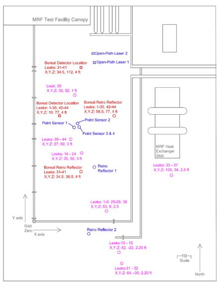
Figure 2.2. Stationary Monitor Leak Locations
