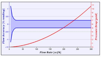
Figure 2.4. Accuracy Chart for the Emerson CMFS010M Coriolis Flow Meter (blue) The mass flux accuracy did not exceed  $\pm 1\%$  of reading during testing. For most test points, the mass flux accuracy was  $\pm 0.25\%$  of reading.
