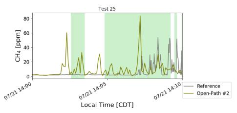
Figure 2.13. Example Test Data from 300-scfh Release for Open-Path #2
