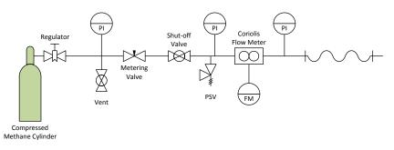
Figure 2.3. P&ID of the Flow Meter Run Used to Control Methane Mass Flux An operator manually controlled the flux using a needle valve and monitored the value using a local flow meter display.
