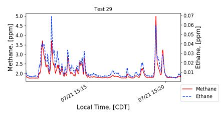
**Figure 2.16. Test of Point Sensor during a 5-scfh Release** The fact that each peak of methane correlates with a peak of ethane suggests that this detection is of a known leak in the facility that contains transmission-grade gas.
