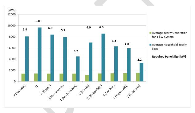
FIGURE 4: Average household loads, generation per installed kW and the PV system size required to cover 100% of household load by climate zone
