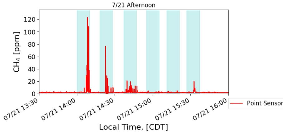
**Figure 2.7. Readings from the Point Sensor Over the Course of One Afternoon**
