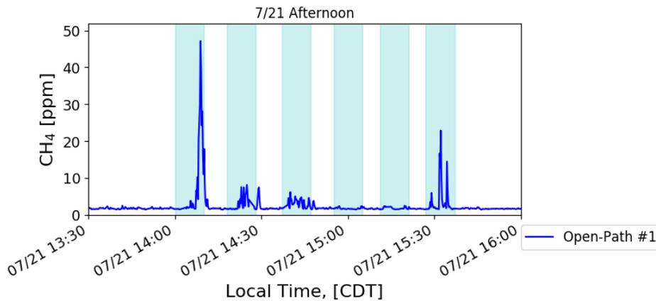
**Figure 2.8 Readings from Open-Path #1 Over the Course of One Afternoon**
