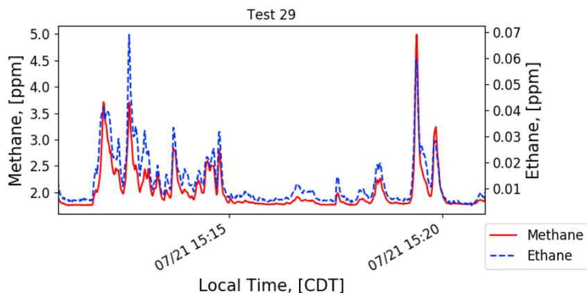
**Figure 2.16. Test of Point Sensor during a 5-scfh Release**
