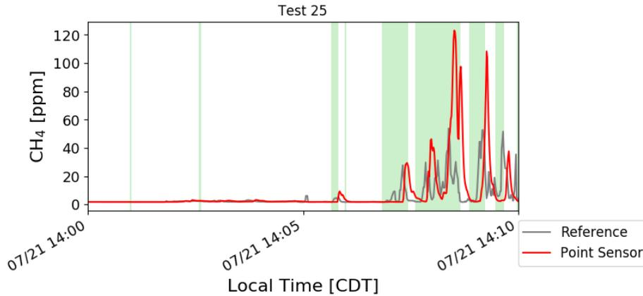
**Figure 2.11. Example Test Data from 300-scfh Release for the Point Sensor**
