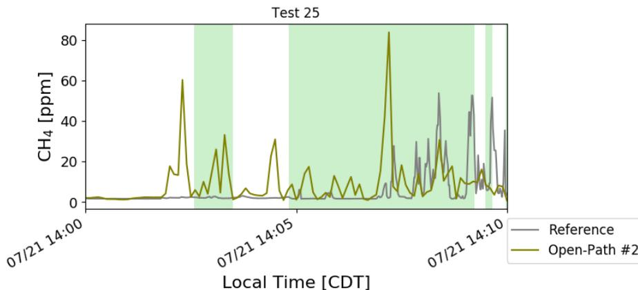
**Figure 2.13. Example Test Data from 300-scfh Release for Open-Path #2**
