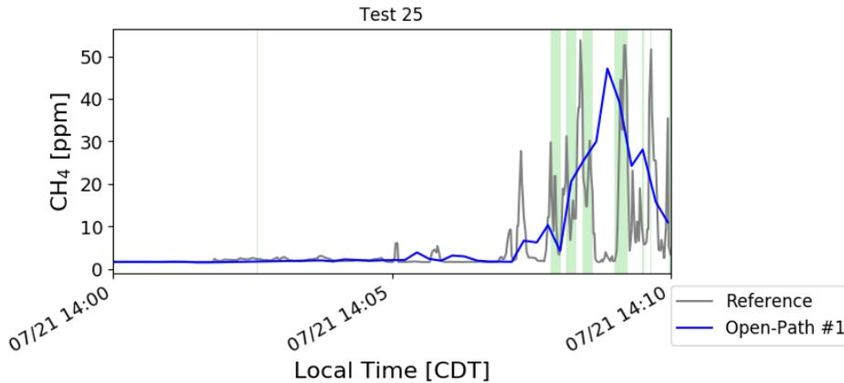
**Figure 2.12. Example Test Data from 300-scfh Release for Open-Path #1**
