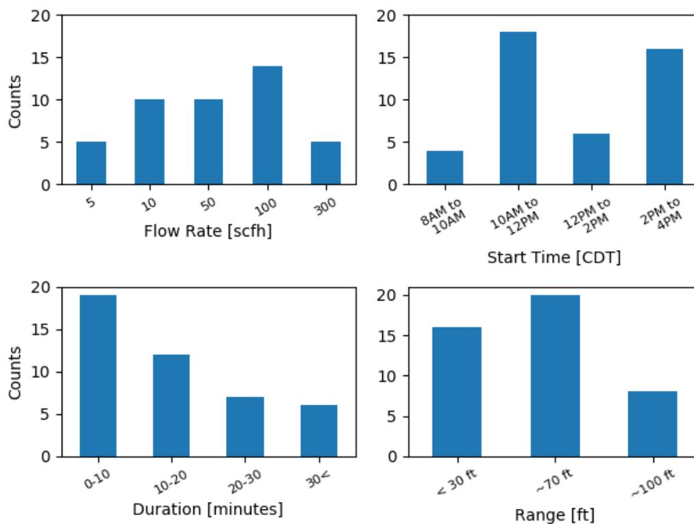
**Figure 2.5 Summary Bar Charts of all Tests Conducted Sorted by Flow Rate (top left), Start Time (top right), Duration of Leak (bottom left), and Leak Range (bottom right)**
