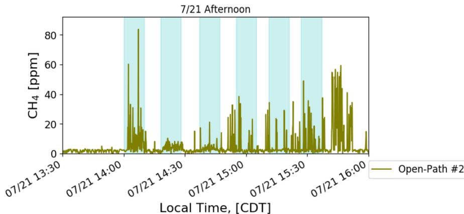
**Figure 2.9 Readings from Open-Path #2 Over the Course of One Afternoon**
