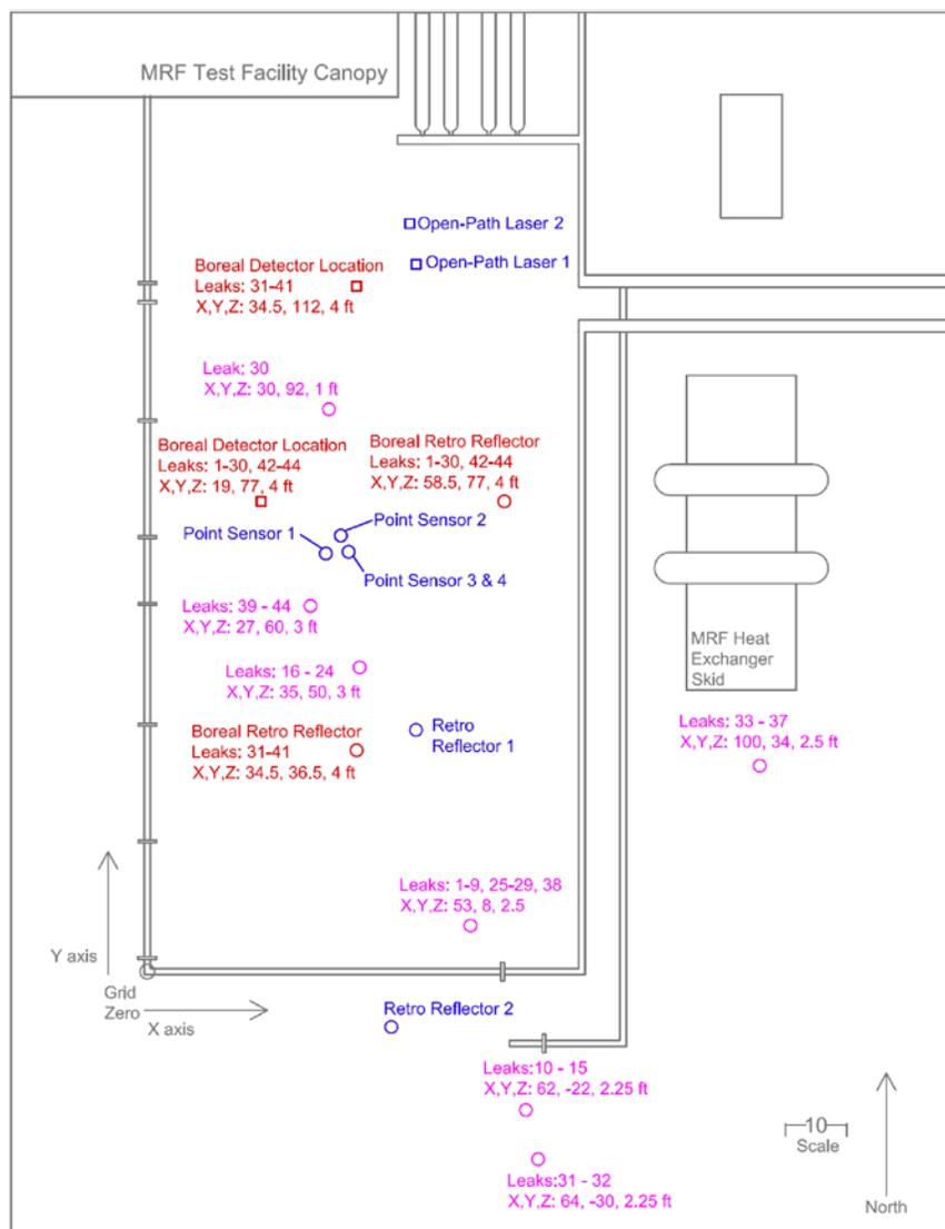
**Figure 2.2. Stationary Monitor Leak Locations**
