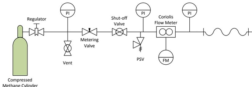
**Figure 2.3. P&ID of the Flow Meter Run Used to Control Methane Mass Flux**
