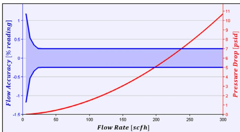
**Figure 2.4. Accuracy Chart for the Emerson CMFS010M Coriolis Flow Meter (blue)**
